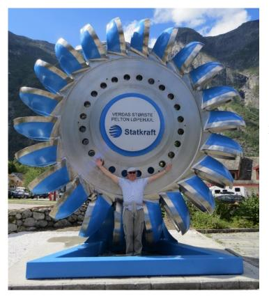
Claimed to be the world's largest electricity generating Pelton Wheel, this example is installed at the Eiriksdal Hydropower Plant in Norway and generates up to 30MW of power.
